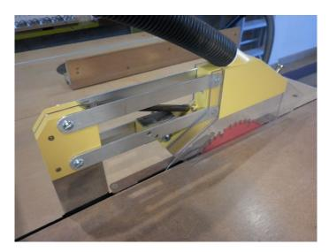
The left side showing the parallel arms and counterbalance spring that are now enclosed inside the Lexan sides. A 32mm outside diameter PVC tube is used instead of a shop vac crevice tool. The space between the Lexan faces is filled with polyurethane foam. The mounting post is the old one with thinner wood faces. Note the 45° cut at the front to provide space for a hole to attach the spring.
