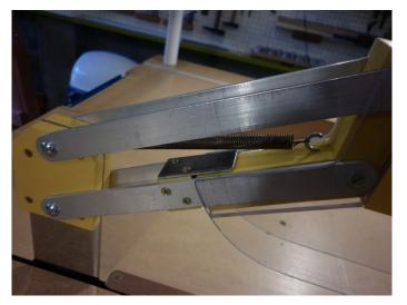
A closeup of the steel plate screwed between the parallel arms. There is a magnet epoxied on the wood core that keeps the Guard up when required.
