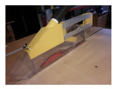
A first view of the Improved Blade Guard. Note the very clean right side and clear view of the saw blade. The Guard body is entirely constructed with 3mm thick Lexan. The only piece of wood being the angled insert to attach the parallel arms and the conterbalance spring end. The rounded entry and exit on the faces work much better than the 45° metal plate of the older version.
